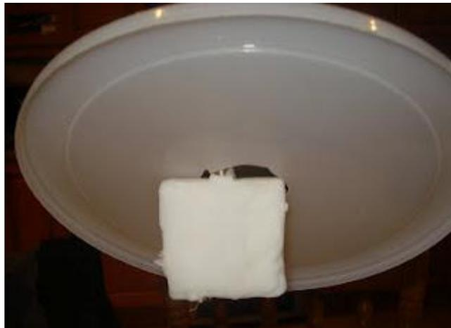
I built the paddle using a template and some polymorph. This is a plastic which can be reshaped when soft.
