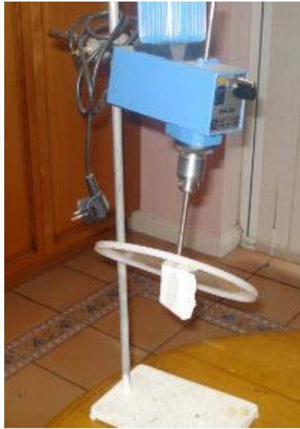
This is a motor used for spinning liquids repurposed. It took me ages to find the right fit for my needs. Most non commercial motors simply over heat after prolonged use or just cut off.
